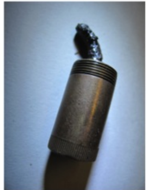
Single-piece oiler for large oscillators (phase2-3, 30-40cm blades)
